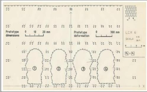
Figure 1. Caverns excavated in chronologic order 1 through 4, showing hysteresis (no reversal of deformation vectors) due to over-closure of the rough fractures, which were under higher normal stress prior to excavation.
