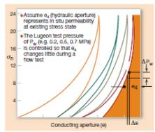
In a 3D sense, the three principal permeability directions (Figure 8), signifying good or partial sealing of at least three sets of joints. The reductions in  $K_{x,y,z}$  and  $K_{x,y,z}$  were more than 1 order of magnitude (between the widely separated boreholes), and deformability (the bulk modulus) also reduced on average by a factor of almost 8.
