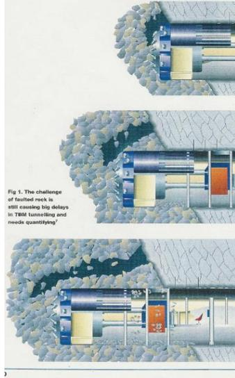
Fig. 1. The challenge of faulted rock in TBM causing big delays in TBM tunnelling and needs quantifying?
