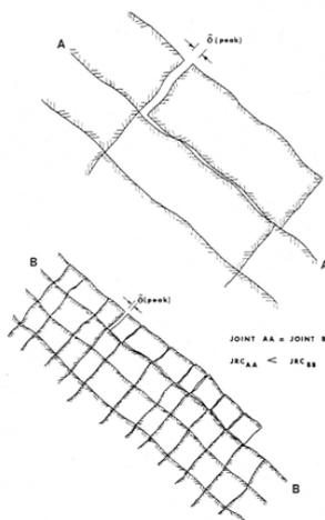
Fig. 1. Scale effect determined by block size, after Barton & Choubey [2].
