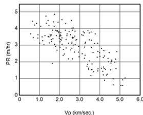
Fig. 1 Declining TBM penetration rate with elevated seismic velocity, due to lack of jointing. The actual advance rate will be a function of opposite effects in the best rock, namely need for frequent cutter change, but little delay for support. Mitani et al., 1987.
