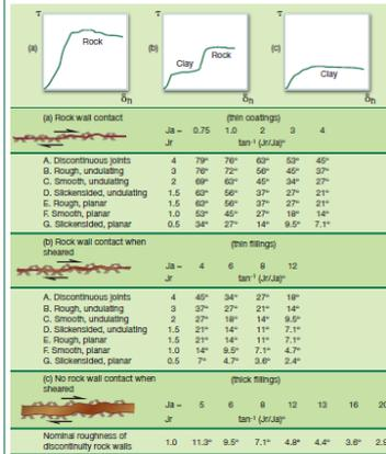
Figure 1. The parameters Jr and Jc are clearly related with 'rock behaviour', despite Goodman's reference to Riedmiller's doubts on this score. Other parameters used in RMR and Q are also clearly related to rock behaviour.
