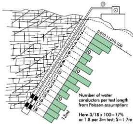
Fig 1: Lugeon testing and zero flow sections as a percentage of the total
