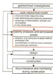
Figure 1: design based on rock mechanical models
