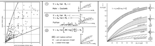
Figure 2. Rock joints do not have cohesion, unless steep steps are sheared through. There is no need to deliberate about whether to ignore cohesion in design. It does not exist. Barton, 1976, 1990, 2006.
