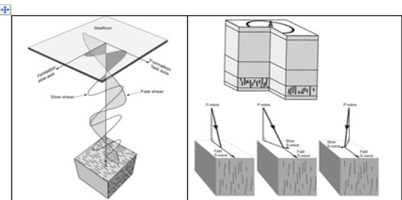
Figures 1a and 1b. The 'one fracture set' conceptual model used in geophysics interpretation of shear wave polarization. This seems to be missing the geomechanics, and production mechanisms needed to explain conductive fractures, and connectivity, at many kilometers depth. *Ervin, Barbed et al., 2004, and Horne, 2003.*
