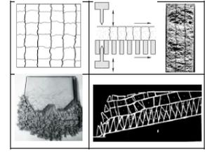
Figure 2. A study in contrast: physical modelling using tension-fracture generation, and numerical modelling using  $\mu$ DEC: this example demonstrates a friction angle for the joints of  $\phi = 20^\circ$ .
