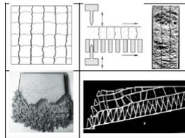
Figure 2. A study in contrast: physical modelling using tension-fracture generation, and numerical modelling using UDEC: this example demonstrates a friction angle for the joints of  $\phi = 20^\circ$ .
