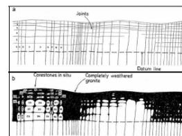
Figure 1. A price has to be paid for tunnel construction too close to the 'dotted line', illustrated from the particular case of weathered granite from Dartmoor, SW England, after Linton (1955) and Fookes et al. (1971). In general, Q-parameters are not easily determined in the Grade V (black) saprolite.
