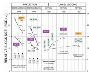
Fig 1 - A demonstration of reduced ROD<sub>20</sub> ratios in a TBM tunnel compared to those predicted. Barton, 2005
