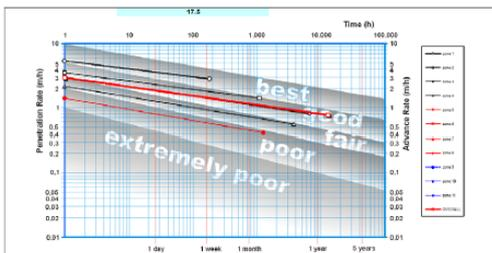
Fig. 1 Example of the  $Q_{TBM}$  prognosis for the 9.6 km North Tunnel (18 months), assuming double-shield excavation, hence the lesser gradients than for open-gripper TBM (see 'open-gripper' adjectives in figure back-ground). Altogether, some 300 rock cuttings were Q-logged to obtain necessary rock mass quality data for the two tunnels. This was combined with the rock-machine data.
