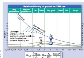
Fig 1 - Penetration Rate (PR) and Advance Rate (AR) as a function of  $Q_{TBM}$ , 2003<sup>1</sup>
