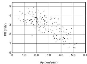
Figure 1: Declining TBM penetration rate PR with elevated seismic velocity. Mitani et al. (1987).
