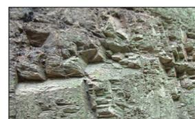
Fig 2 - An exposure of the Brisbane NFB meta-sediments that illustrates the importance of the combined ROD<sub>20</sub>, ROD<sub>20</sub>,  $J_n/J_v$  on block release. PR and AR may be affected in opposite directions: easier boring, subsequent delays.
