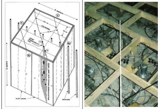
Fig. 1 The ONWI/TerraTek heated block test for testing the coupled HTM (hydro-thermo-mechanical) behaviour of a jointed crystalline rock. Mean jointing trends are shown. A range of strain and deformation gauges are seen. (Hardin et al. 1981, Barton, 1982).
