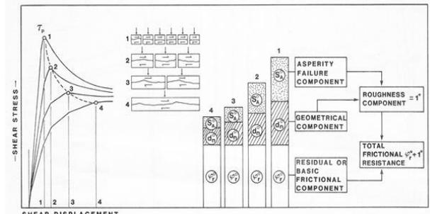
Figure 1. Scale dependent properties of rock joints, after Bandis et al. 1981.
