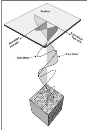
Figure 1. The conventional interpretation of shear-wave polarization, with the fast axis caused by one set of stress-aligned fractures or by microcracks. From Barton et al. (2004).
