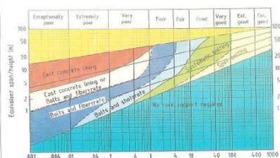
Figure 1. Simplified diagram for design of rock support based on the Q-system (Grimstad et al., 1986).
