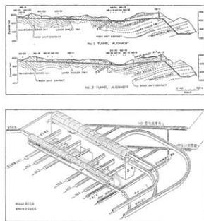
Figure 1 - The Mingan pumped storage project in Taiwan. Powerhouse axes were finally perpendicular to the strike of the bedded sandstones, siltstones and bedding plane faults. (Liu, Cheng and Chang, 1988/Taiwan Power Company and Sinotech Inc.).
