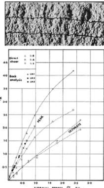
Figure 1. Over-closure (OC) ratios of 8:1, 4:1 and 1:1 (conventional) prior to direct shear testing of rough tension fractures. Barton, 1972. An example of the model tension fractures, and their surface roughness is also shown. 'Back-analysis' refers to the model slope failures.
